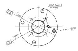
Detailed drawing of base mounting face
