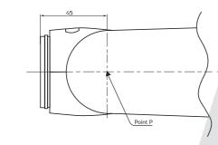
Built-in A/F 2D camera Pixel: 2.07 Megapixel
